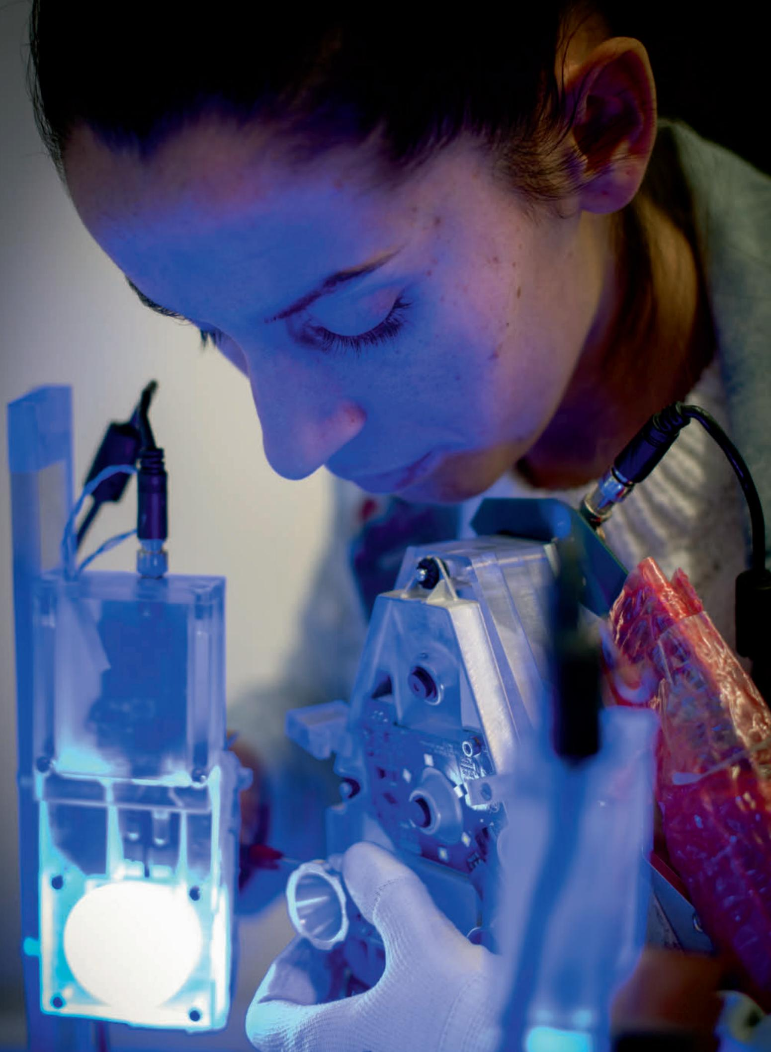
Another example: In the automotive industry, which is today undergoing a major transformation, handheld and wireless 3D scanners are a valuable and easy-to-use tool for reverse engineering design. With some basic training, the engineer is able to digitally reproduce components with very high accuracy. This scanning solution can be integrated into existing design workflows or used independently and is compatible with existing CAD/CAM programmes.
