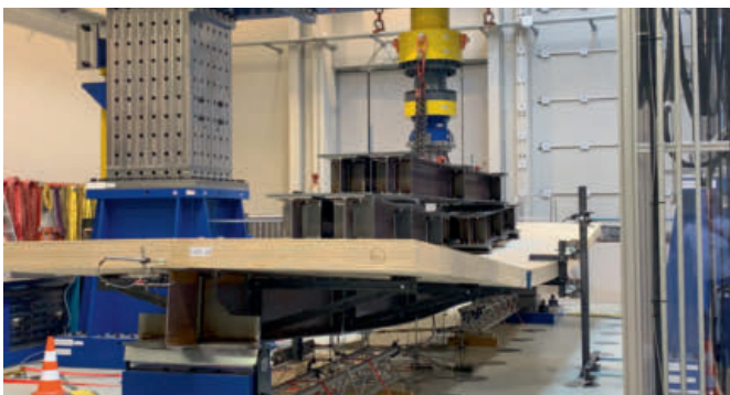
Large scale bending test in the laboratory of structural engineering of the University of Luxembourg
